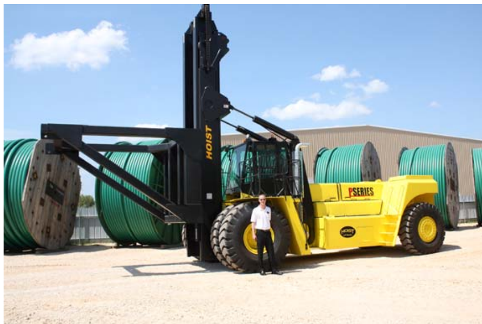
Hoist Liftruck will provide the Alabama State Port Authority with two P-Series P1000s (100,000-pound capacity), similar to the P1100 (110,000-pound capacity) pictured above. Hoist Liftruck is one of the top manufacturers of large-capacity forklifts in the United States.
