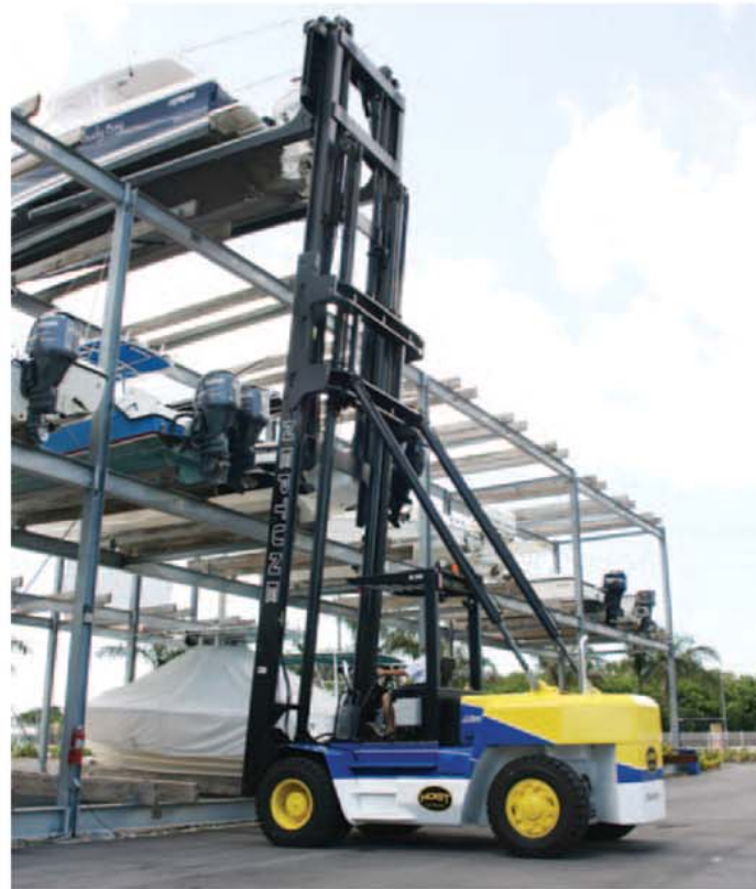
Pictured: The Neptune Series handles boats weighing as much as 55,000 pounds, transporting them in and out of rack storage.
