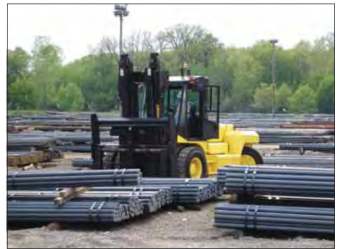
A Hoist P-series truck handling steel bar and (below) close-up of access arrangement
